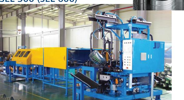
The Super Elbow Line, Type 300 SEL (SEL 600) was especially designed for the production of elbows in a continuously process. The manual production of these elbows needs a lot of time and effort. With consistently high quality in production, this machine saves with its autonomous functioning an enormous amount of time.
